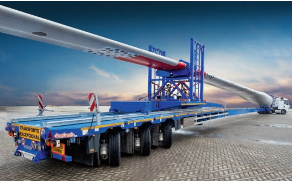
The Super Wing Carrier for the transport of gigantic 65-metre wind turbine blades.
