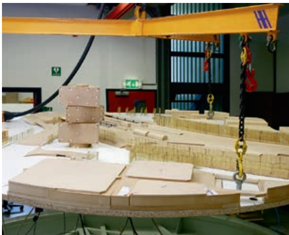
Model of a location with buildings is lifted into the wind tunnel
